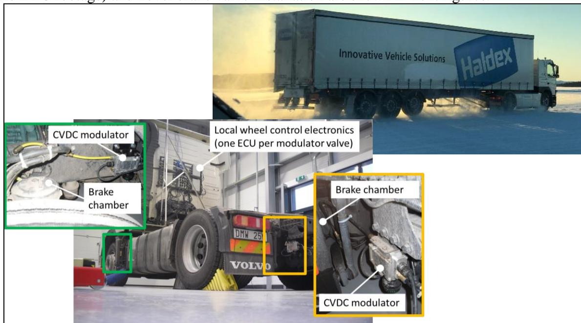
The research project investigates if vehicle control and wheel brake actuator control can be developed in a modular way, with strict standardised signal interface between the controls. Chalmers participates in project and develops tyre characteristics estimator for actuator controls. Two concepts are investigated, “recursive estimator” and “extreme-seeking estimator”.
