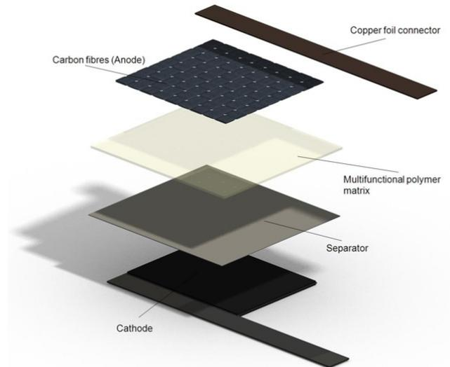
Figure 1: Schematic illustration: Structural battery laminate
