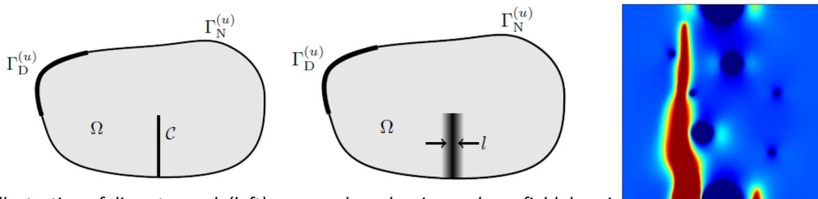
**Figure:** Illustration of discrete crack (left), smeared crack using a phase-field description (middle), and numerical simulation of crack-propagation (under monotonic loading) in a heterogeneous medium (right). (Bharali et al. 2020)
