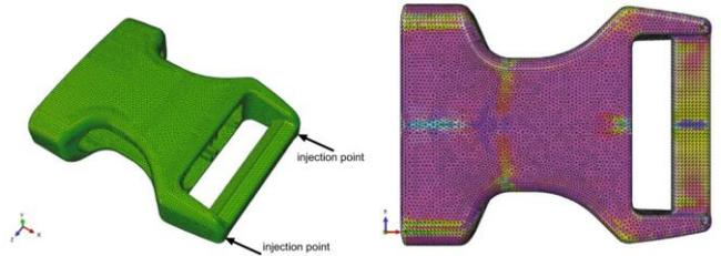
Figure 1: Injection molded quick release buckle socket: (a) finite elements mesh, (b) fiber orientation distribution (Köbler et al. (2018) Comput. Mech. 61:729–750)
