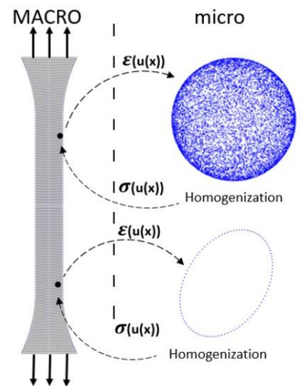
Figure 2: Schematic representation of the coupled multi-scale model for short fiber composites.
