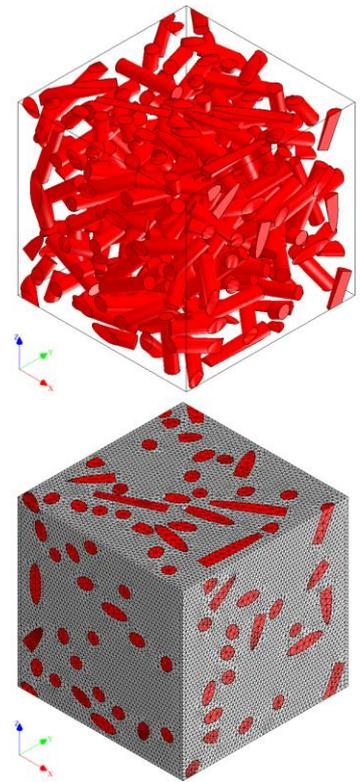
**Figure 1:** An RVE of a short fiber composites and its spatial discretization [1]
