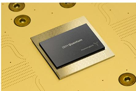
**IBM reaches quantum volume of 64.** In August, IBM announced having achieved the company's highest quantum volume this far. Combining a series of new software and hardware techniques, IBM upgraded the performance of one of its newest cloud-accessible 27-qubit chips to a quantum volume of 64. The higher the quantum volume, the more complex the tasks a quantum computer should be able to solve.
