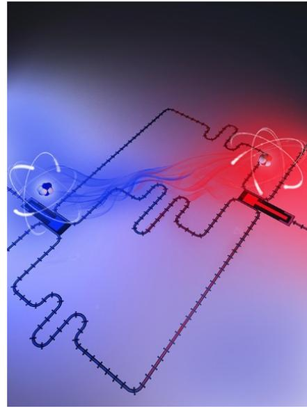
*Two superconducting qubits acting as giant artificial atoms by coupling to a waveguide at multiple points.*
