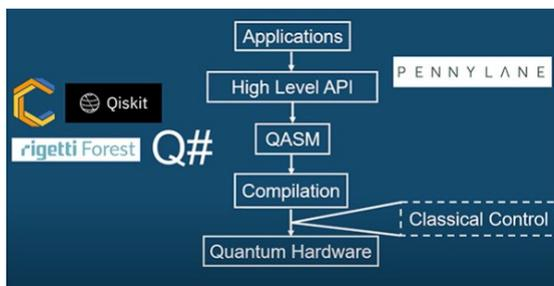
Nowadays, there are several powerful and useful tools for developing quantum software, for example Qiskit, Cirq, and PyQuil to name a few. However, these tools are generally developed by and for theorists, and therefore focus high up in the computing stack for implementing quantum algorithms.
