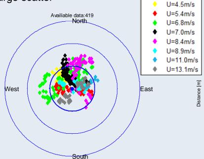
Wind speed between 4.5 – 13 m/s at the time of ice release
