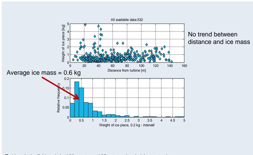
Turbines in the field study had 90 m rotor and 95 m tower (no de-icing system)
