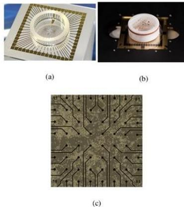
**Fig. 1.** (a) A generic MEA. (b) A MEA with a neuronal culture. (c) Microscopic image of culture with visible neuronal structure formation.
