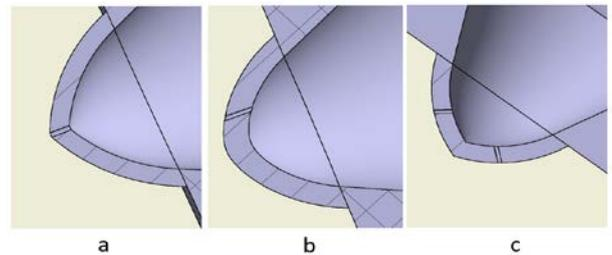
Figure 2. Nozzle geometries a) Single hole, On-axis orifice, Parallel nozzle and orifice axes, b) Single hole, Off-axis orifice, Parallel nozzle and orifice axes, c) Double hole, Deviated orifice axes
