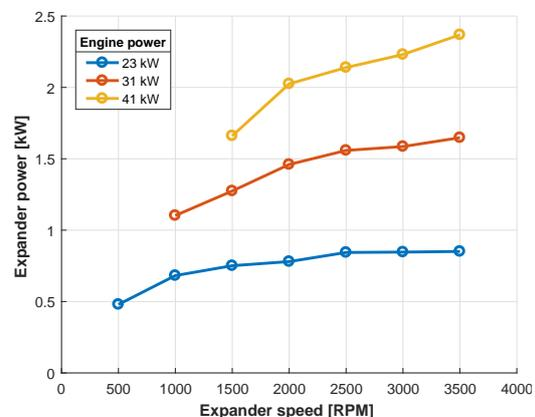
Figure 2: Expander power vs. expander speed for different engine operating points.
