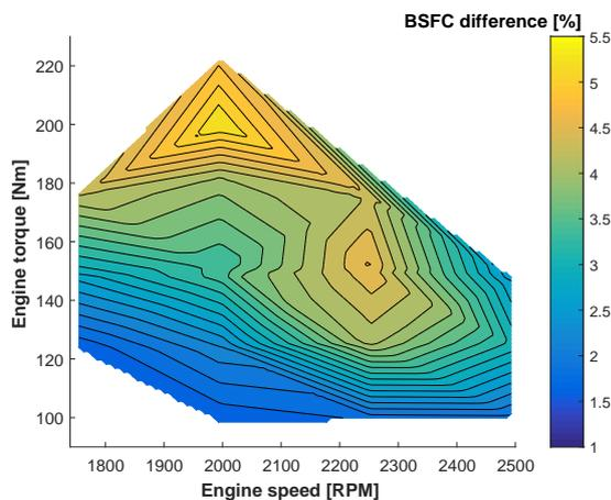
Figure 1: Difference in BSFC with and without the expander coupled to the engine.
