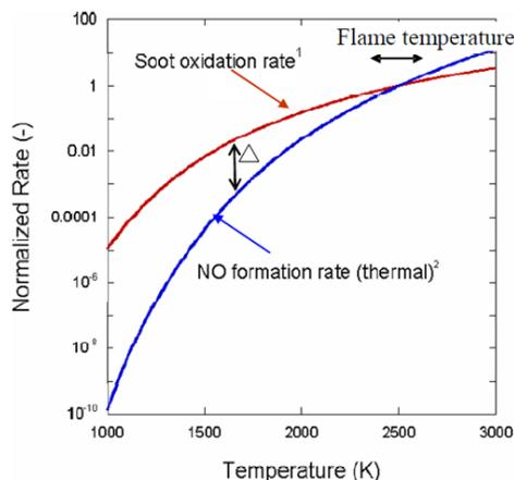
Figure 1: Reaction rates for the oxidisation of soot together with oxygen ( $O_2$ ) and the formation of nitrous oxides ( $NO$ ) as function of the local flame temperature<sup>1</sup>.
