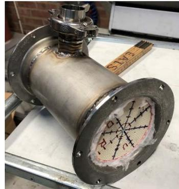
Figure 1 A simplified EATS with an inert monolith cased in a “reactor” with a deviating flow and potential thermal gradients.
